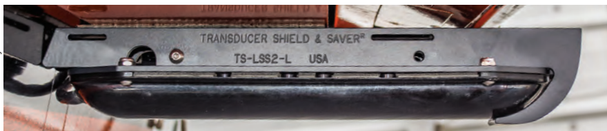
A transducer shield is good insurance for any skinny water where wood cover, rocks or grass might cause damage.
